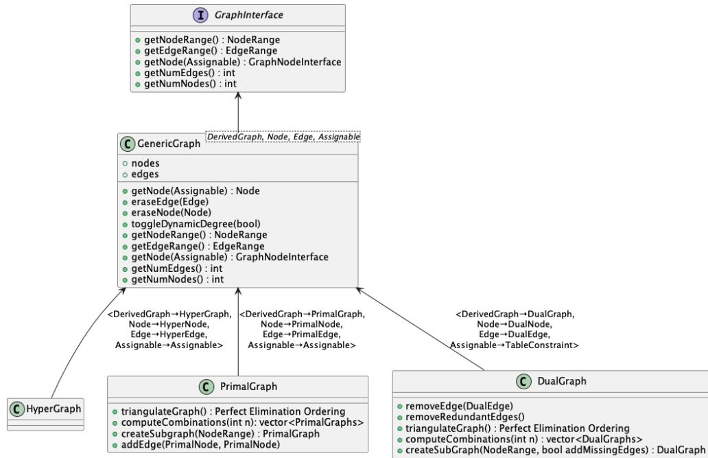
Figure 3.3: Class diagram of STAMPEDE’s graph structures.
